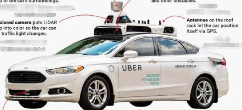
LIDAR modules on the front, rear, and sides help detect obstacles in blind spots.
